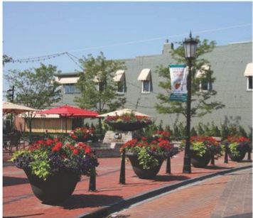
Movable bollards between fixed planters
